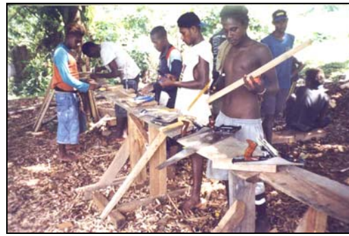
Joinery class session: Year 1 students during a practical lesson on how to mark and cut chair legs
